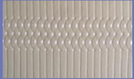
Jersey rib-structure pattern in gore technique.
